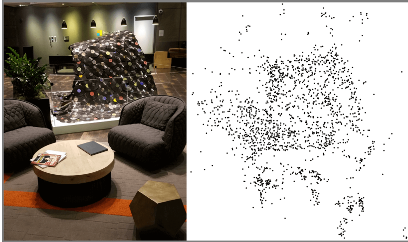
Figure 3.1: Real-life environment and the resulting sparse point cloud (source [61])
